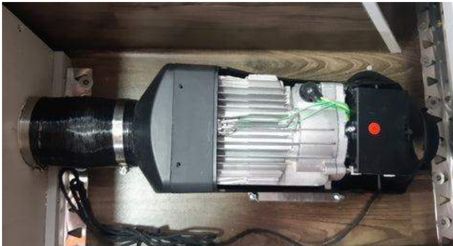
Photo: Clean Diesel Heater Combustion Chamber
