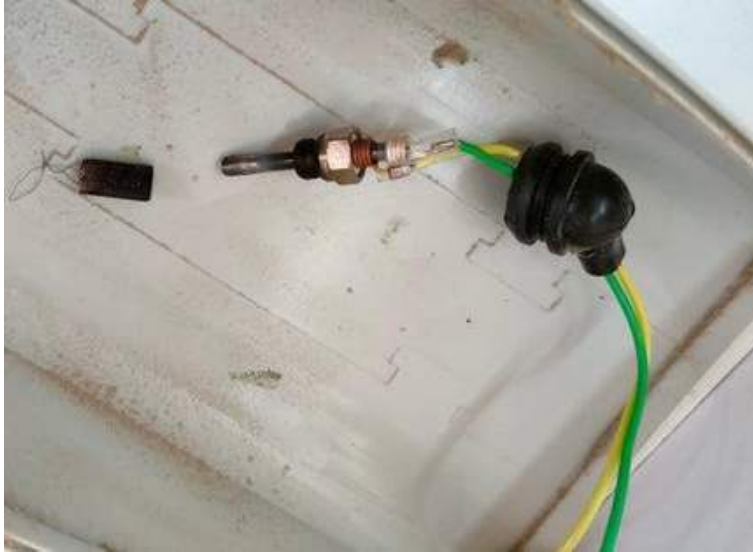
Photo: Used glow plug screen with carbon built up.
