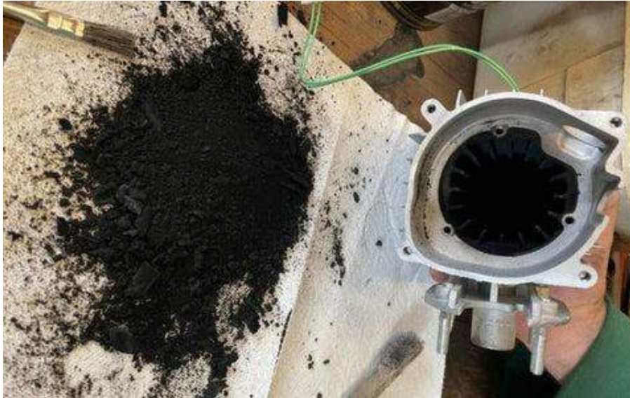
Photo: Diesel Heater Combustion Chamber with Excess Carbon Build-up. Cleaning Recommended.
